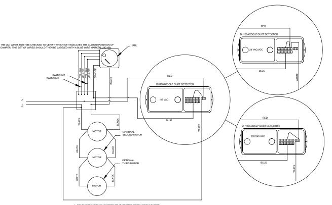
1. CONDUIT RUNS WHICH EXCEED 72" MUST HAVE GREEN GROUND WIRE. 2. FLEX CONDUIT MUST BE SECURED WITH A CONDUIT CLAMP (48298) WITHIN 12" OF CONDUIT TERMINATION AT THE HANDI-BOX OR ACTUATOR. CONDUIT RUNS MUST ALSO BE SECURED ALONG SLEEVE AT A MAXIMUM OF 24" ON CENTER.
